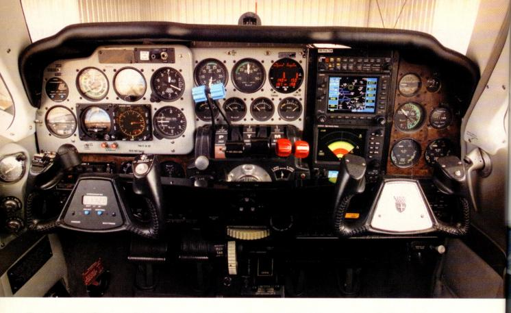
Beechcraft carried over to the Baron the layout of the Beech 18 panel, where the throttle levers were in the middle of the quadrant, giving pilot and copilot equal access to the go-levers.
